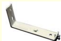
WB-17-5P-100 Inst. Bracket, with screw, For 127mm system WB-17-5Z-100 Painted, PLATED, W=2.0mm,L=84mm
